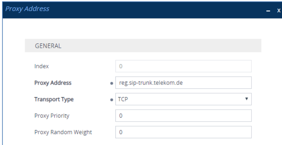
Figure 4-17: Configuring Proxy Address for DTAG's DLAN SIP Trunk
